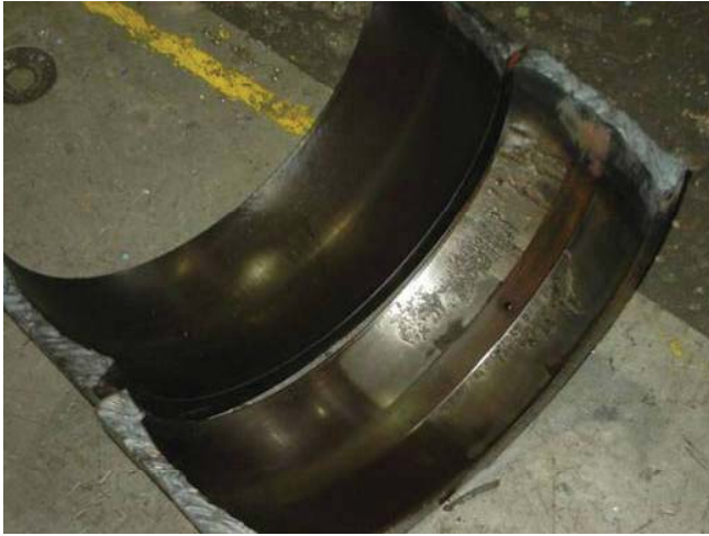
visual inspection confirms drive.mon alarm
